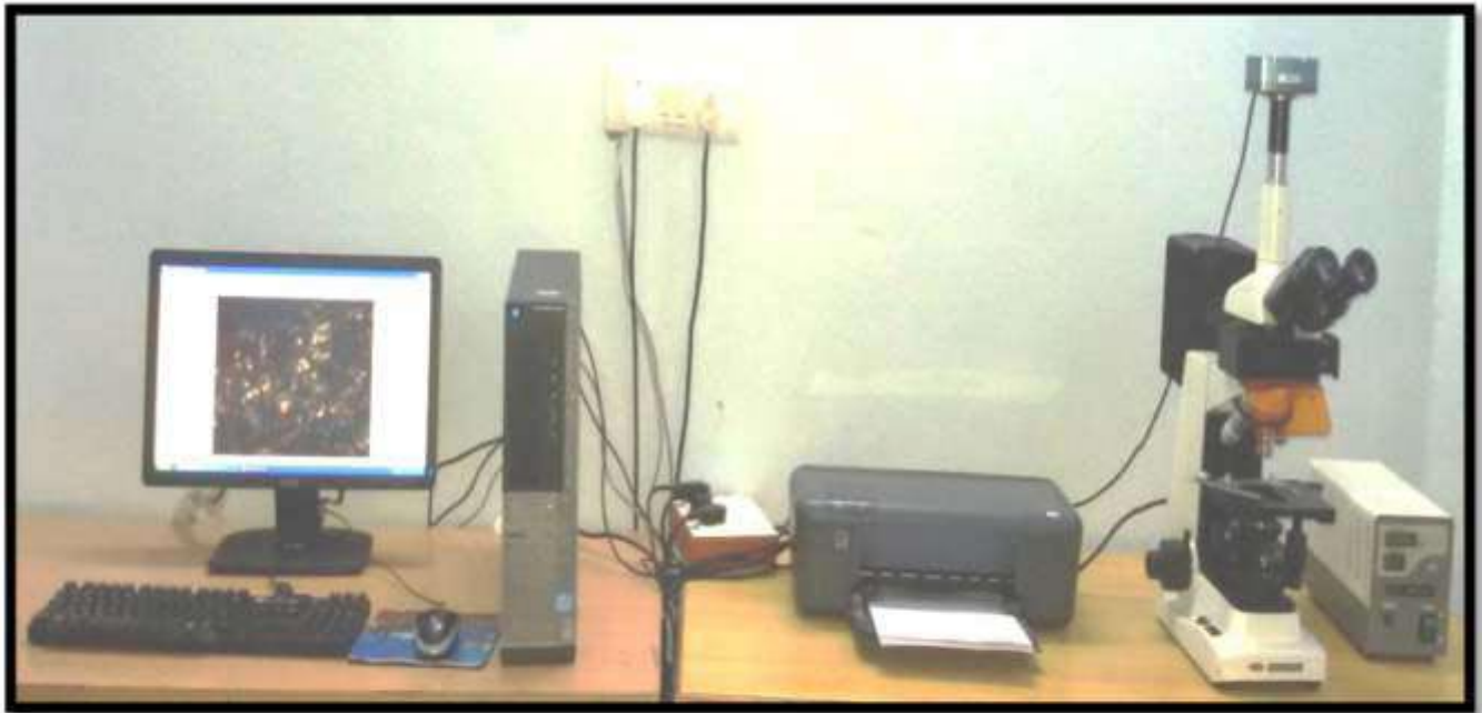
Photograph showing Trinocular Research Microscope (Lynx microscope, Lawrence & Mayo) with camera
